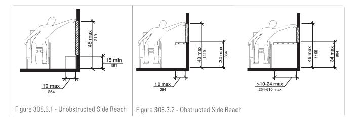
308.3.2 Where a clear floor or ground space allows a parallel approach to an element and the high side reach is over an obstruction, the height of the obstruction shall be 34 inches (865mm) maximum and the depth of the obstruction shall be 24 inches (610mm) maximum.
