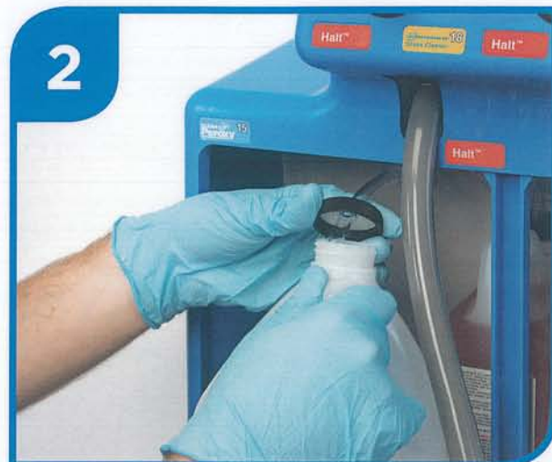
2 Remove empty container and unscrew cap
