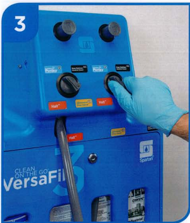
Select bucket fill product by turning dial to desired product
